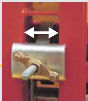
Move element sideways By releasing the Strongback Connector U 100-120.
