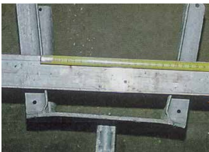
Cross Forkhead ■ bent head plate > 5 mm
