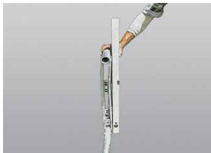
T-Frame UVT ■ bent ■ assembly of decking is possible ■ damaged at one point but no cracks in the welding seam
