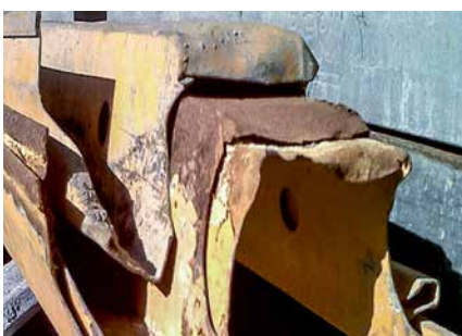
Toeboard Steel UPY ■ heavy deformation of the toeboard edges
