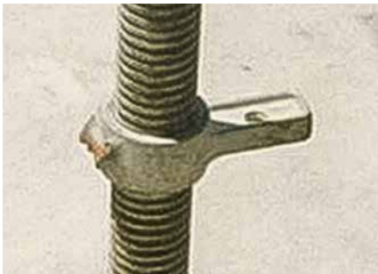
Spindles UJB / UJS / TR 38-70/50 ■ wingnut is defective
