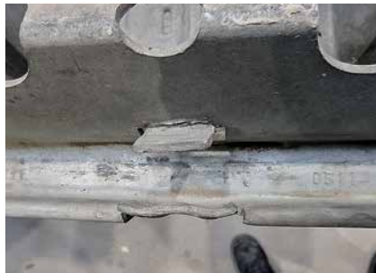
Scaffold Decks UDS ■ lug of the lift-off prevention is broken
