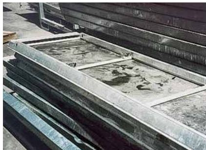
Access Deck UAL ■ damaged ladder ■ hole in deck ■ snap fastener is damaged
