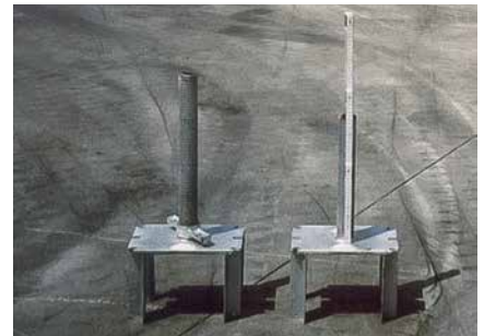
Cross Forkhead ■ sawn off spindle
